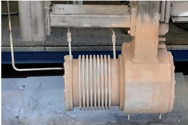
Protecting bellow of high temperature tight bearing with boride layer for immersed roll in galvanising line
