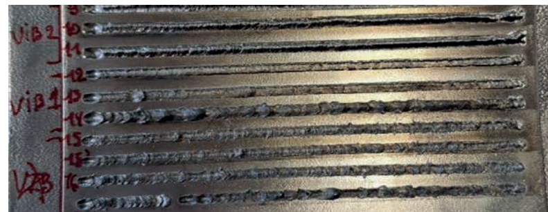
Study on joining additive printed components - Lap-joint electron beam welding trials, testing different welding parameters with and without vibration of the beam
