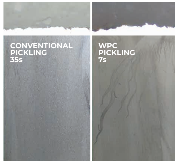
Potential for enhancing pickling operating by WPC pickling: sample pickled with WPC technology for 7s results in the same surface state as the sample pickled for 35s in the reference deep tank conditions.
