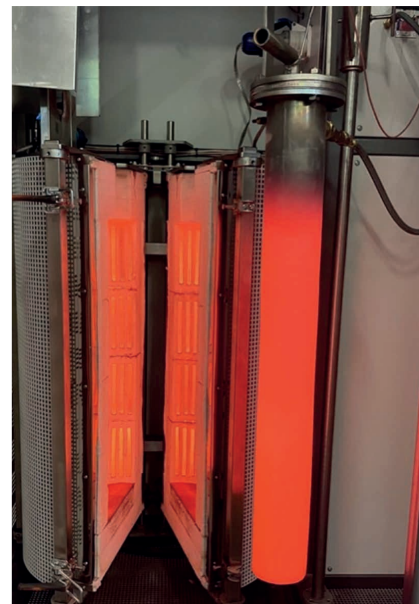
Lab furnace initially designed for ISO characterisation of Blast Furnace Ferrous Burden transformed for Direct Reduction shaft simulations
