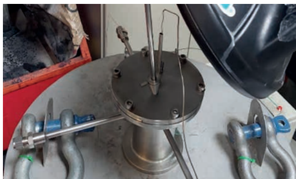
Electrochemical corrosion testing at very high temperatures and under controlled atmospheres
