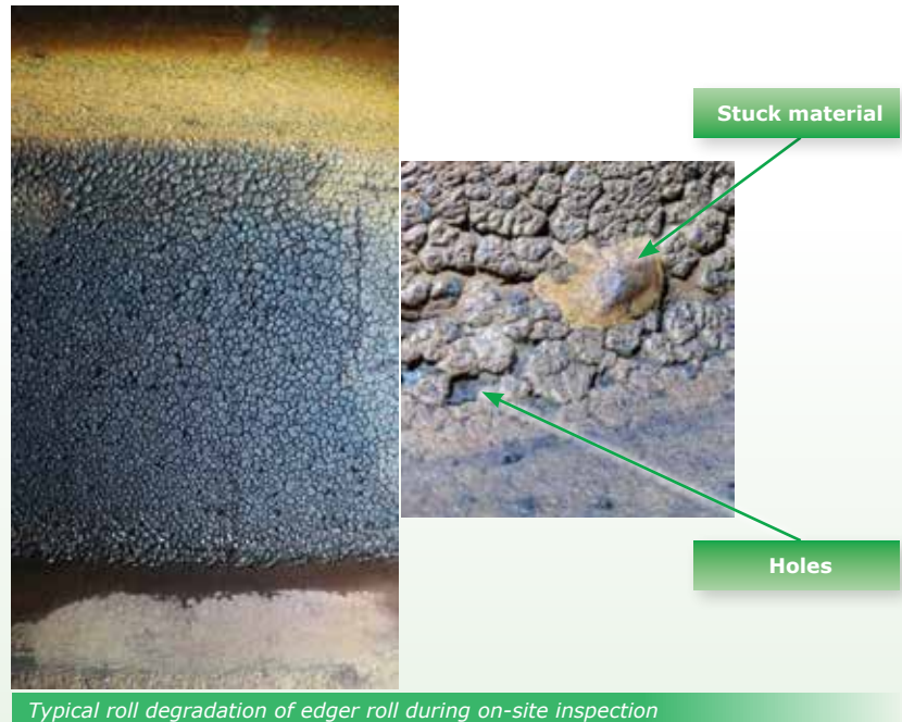
Typical roll degradation of edger roll during on-site inspection
