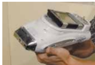
Handheld XRF device used for (roll) oxide thickness measurements
