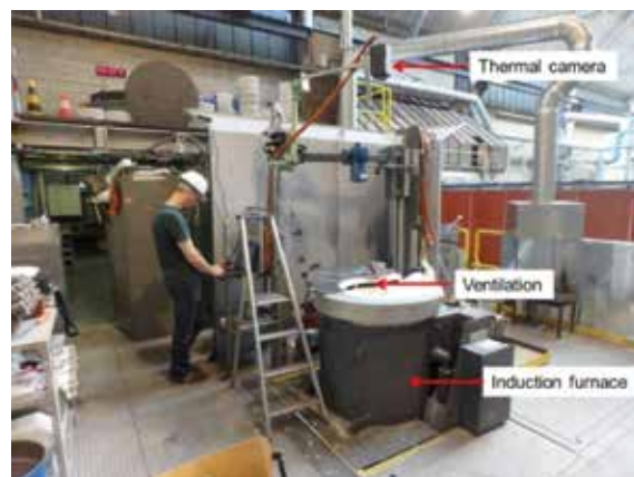
Study of the dissolution of briquettes in the HIsarna process
