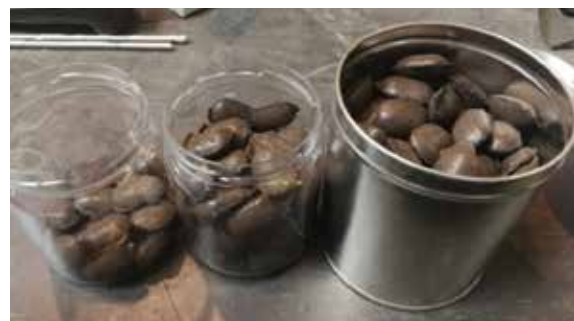
Micro granules and briquettes prepared from BOF sludge and EAF dust for remelting in HIsarna furnace
