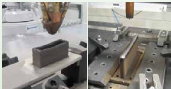
Definition of optimised deposition parameters for high strength steels with laser metal deposition (left) and WAAM (right)
