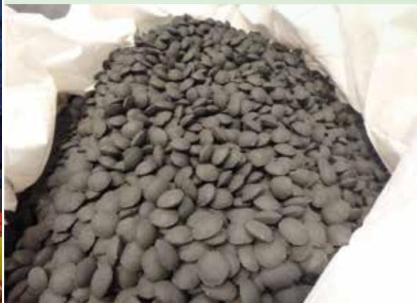
Production of 5 tons of briquettes with by-products from industrial partners to be used as alternative ores
