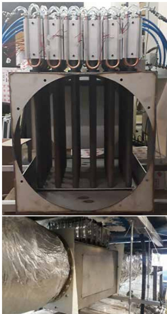
Thermoelectric testing unit (up: internal view, down: installed on an off-gas duct)
