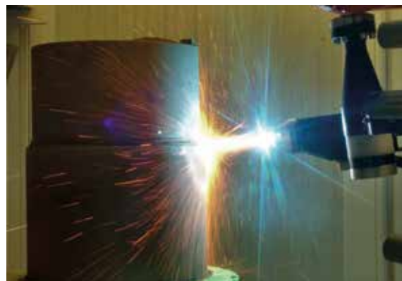
Thermal spray of NiCr coating on 3D parts as alternative to electrolytic Cr treatments
