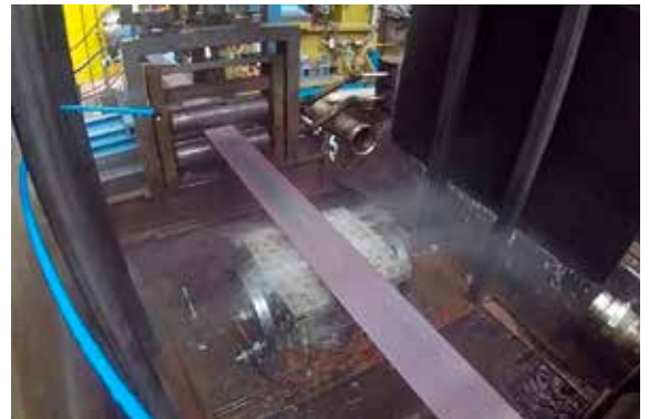
Smart cooling actuator tested on pilot line
