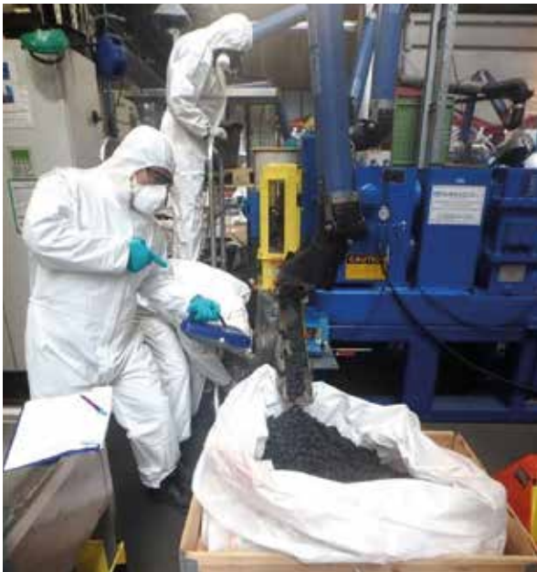
Production of 5 tons of briquettes with by-products from industrial partners to be used as alternative ores
