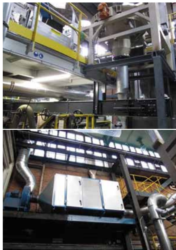
Pyrolysis platform: New big bag unloading station with conveyor (up), new filter (down)
