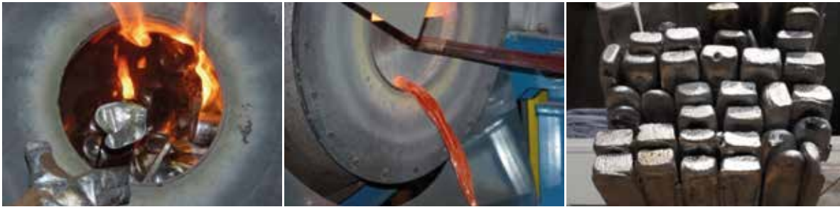
Light Al-packaging re-melting – Rotary tilting furnace – cast Al ingots from recycled Al
