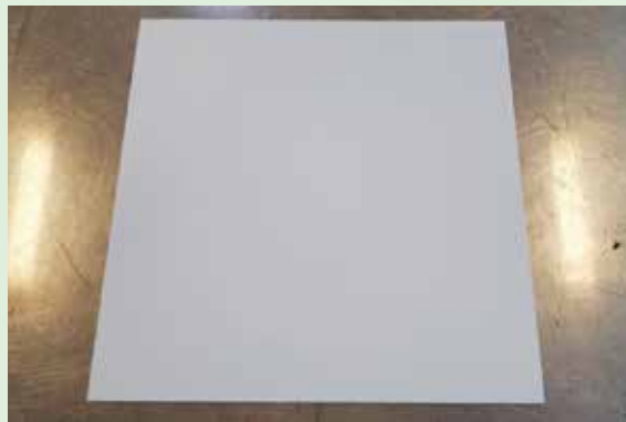
Sol-gel coating on metallic substrate applied by electrostatic spray
