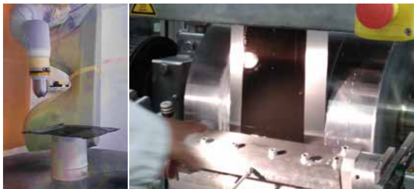
Robotic spray (left) and wet roll-to-roll coating line (right) in clean room environment used for the upscaling of the battery production method without the use of toxic solvents
