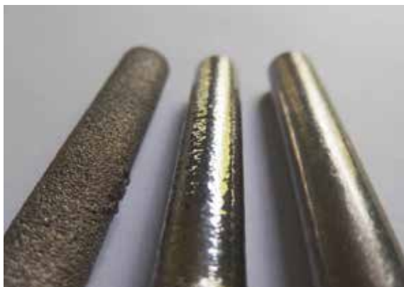
Surface finishing of coupons for aerospace applications. From left to right : reference sample, surface processing 1 and surface processing 2
