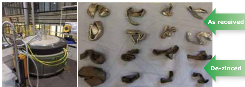
De-Zincing of scrap in the thermal pre-conditioning furnace
