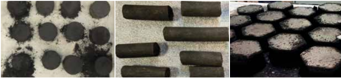
Agglomerates produced with the same mixture of \text{MnO}_2 and spent active carbon using 3 different technologies, for recycling into a Cupola furnace
