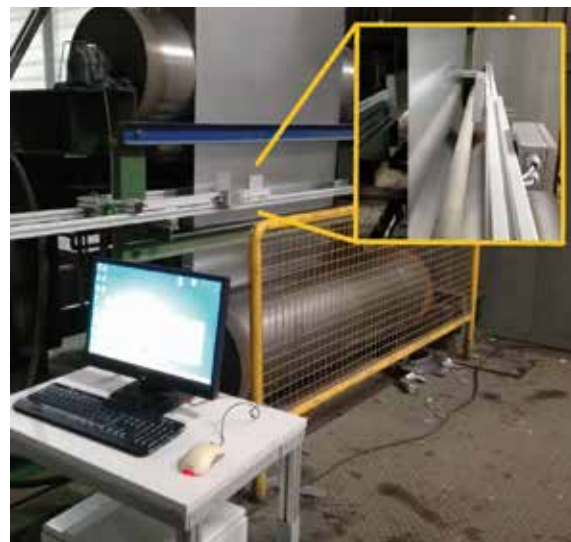
Prototype of the austenite measurement system installed in industrial galvanising line
