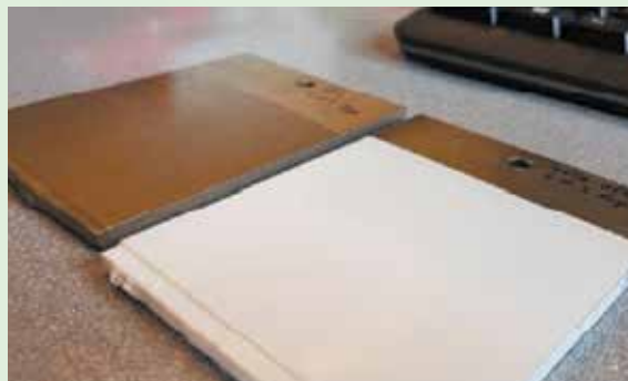
Samples with varnish and ceramic coating applied after electropolishing
