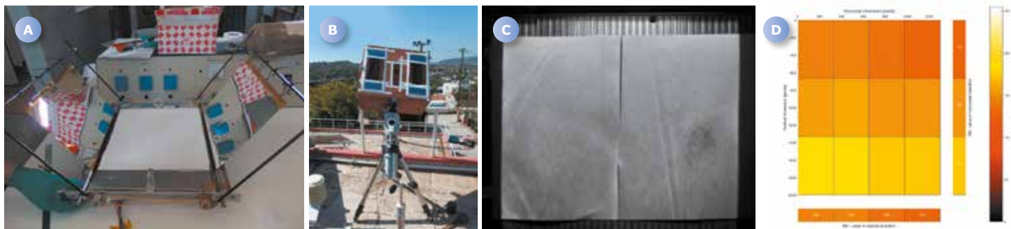
A Solar Concentrator Prototype after assembly - B Laboratory light reflection trial - C Result of light reflection trial D Result of image analysis of the laboratory light reflection trial.
