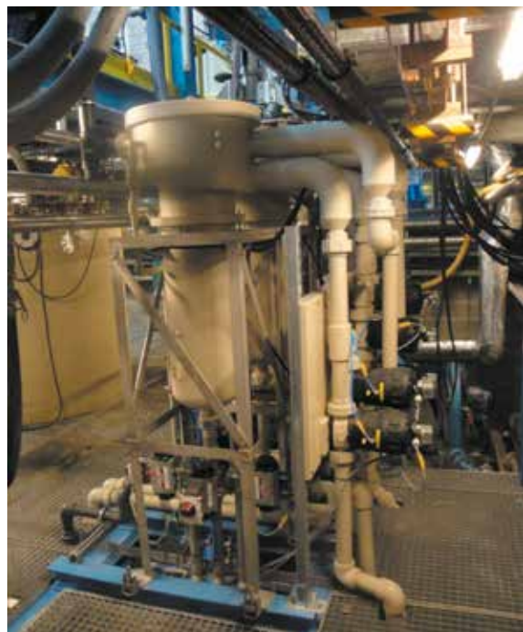
The new electroplating module installed on CASTL pilot line and dedicated to 3D objects
