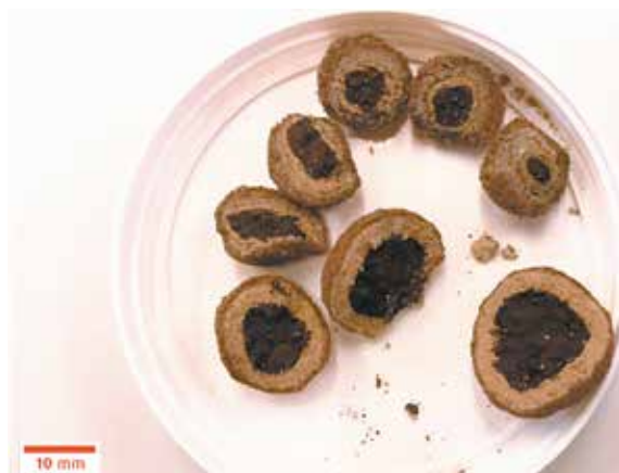
Dual material pellets
