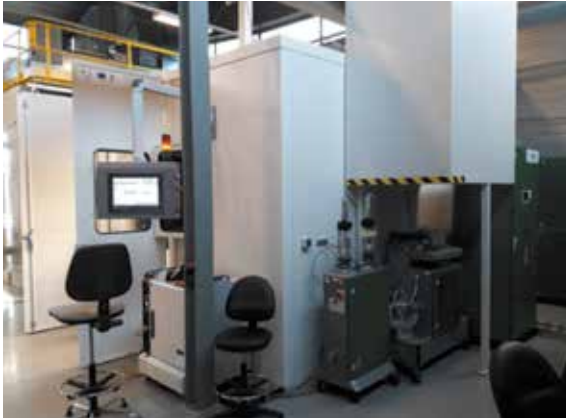
Thermal spray booth for application of thick coatings on 3D parts
