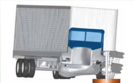
Numerical simulation of crash test for safety barrier design
