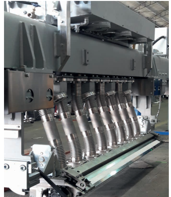
CrossBowMeter: measurement of the shape and vibrations of the strip just above the wipers in galvanising lines.
