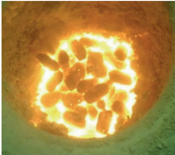
Melting in steel bath of self-reducing briquettes produced from waste Al-powder from additive manufacturing.
