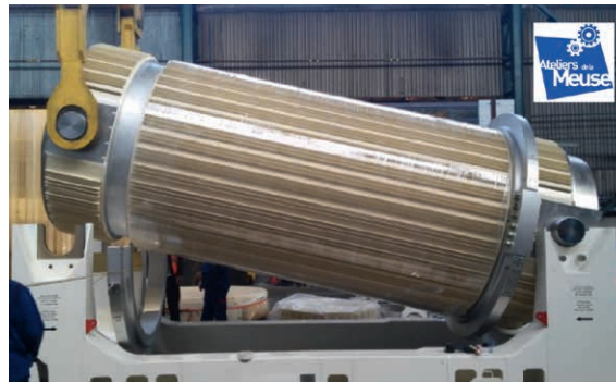
NDT inspection of packaging for nuclear waste.
