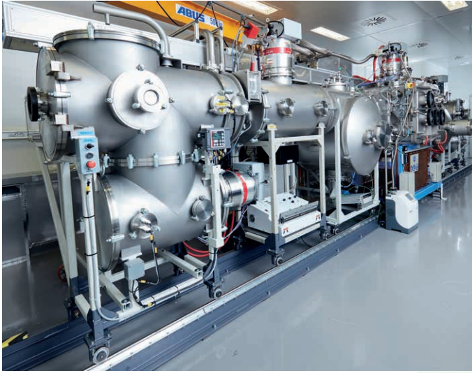
Roll-to-roll pilot lines supporting the energy projects (left: vacuum, right: wet coating).
