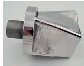
Shiny surface of pump rotor printed by LMD after surface finishing.
