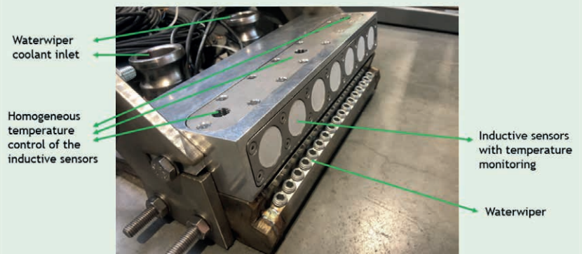
New wiper concept: waterwiper with integrated roll profile measurement sensor ready to be implemented in cold rolling pilot line.
