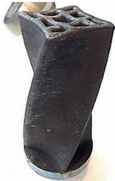
Demonstration of 3D printing of a pump rotor in 17-4PH.
