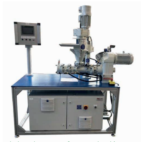
Extruded agglomerates from steelmaking by-products – Stiff vacuum extruder.
