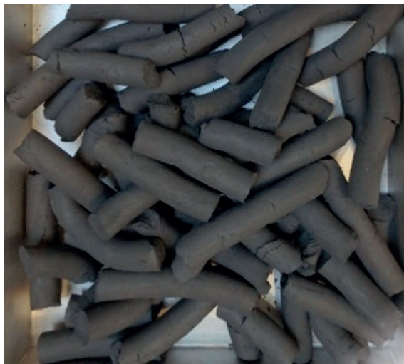
Extruded agglomerates from steelmaking by-products – Stiff vacuum extruder.
