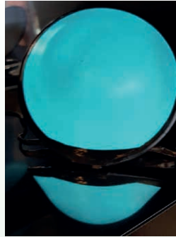
Electroluminescent stack on 3D-preformed steel plate.
