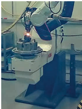
Demonstration of 3D printing of a pump rotor in 17-4PH.
