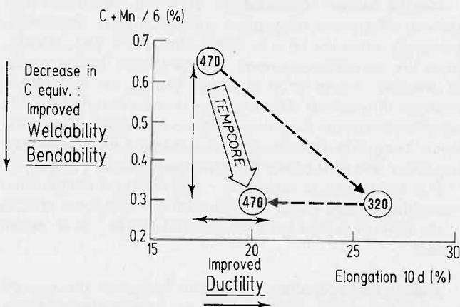
Figure 6. Weldability and ductility properties of Tempcore rebars
