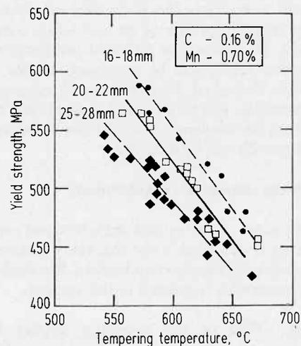
Figure 4. Example of yield strength/tempering temperature relationships
