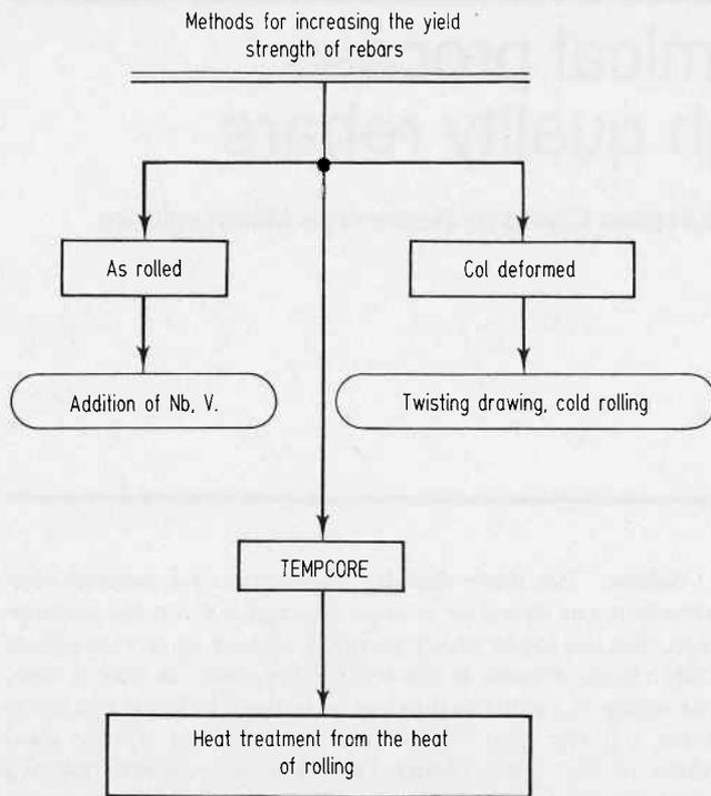
Figure 2. Methods for increasing the yield strength of rebars
