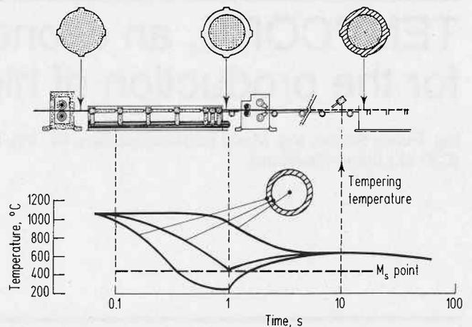
Figure 3. Schematic representation of the Tempcore process
