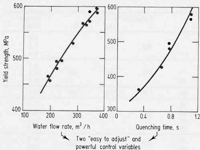
Figure 5. On line control of Tempcore
