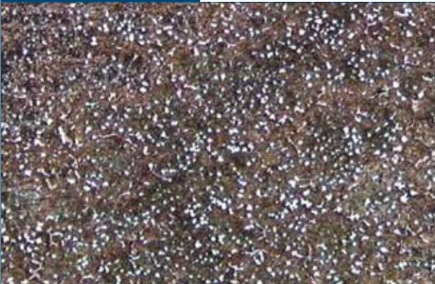
Fully heat-treated microstructure of RTB7 (HSS5). hfw = 2,000 μm.
