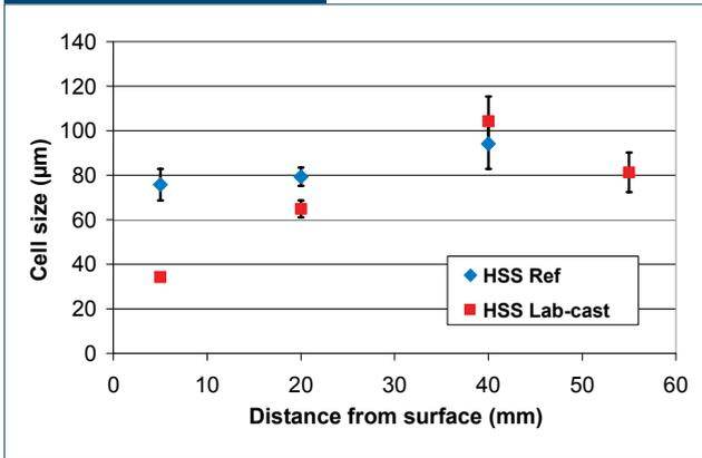
Cell size measurements according to ASTM-112, for high-speed steel (HSS) reference (roll) and HSS test block material.
