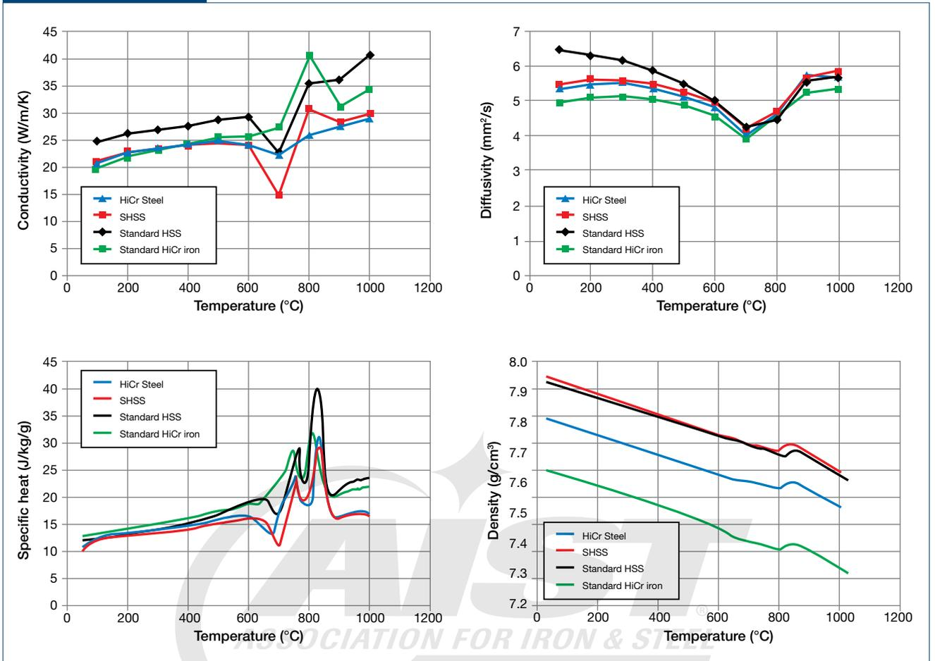
The thermophysical properties of HiCr steel and SHSS compared to standard HSS and HiCr iron material.
