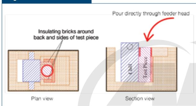
The rectangular test block (RTB) molding.
