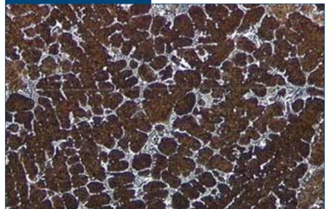
Hi-Mo HSS roll microstructure. hfw = 2,000  $\mu$ m.
