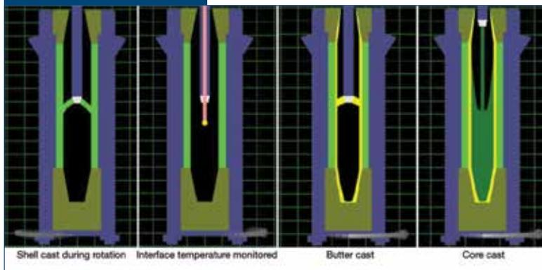
A schematic of the vertical centrifugal casting process.
