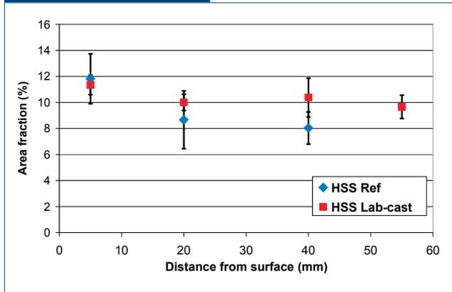
Area fractions of primary carbides as function of radial depth in for HSS reference (roll) and HSS (test block) material.
