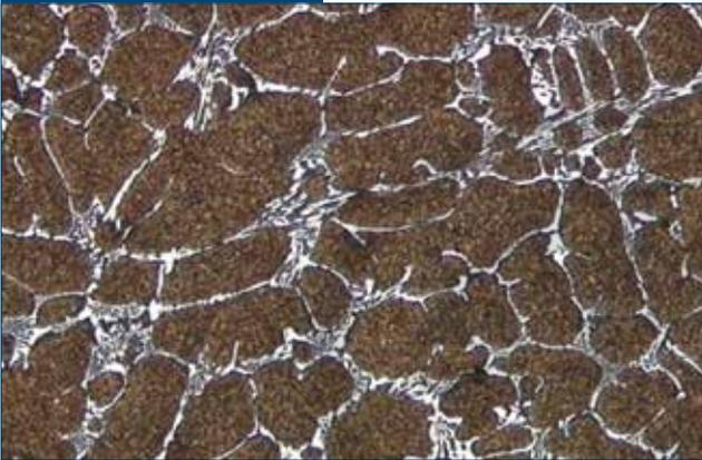
HiCr steel microstructure. hfw = 2,000  $\mu\text{m}$ .
