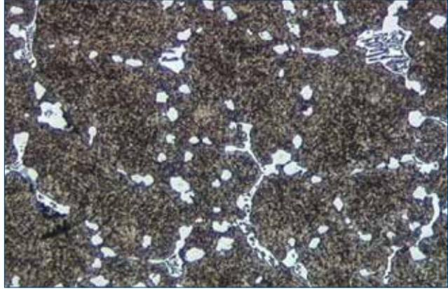
HSS6 microstructure. hfw = 500 μm.
